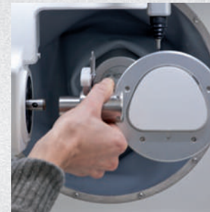
Easy change of the blank holder for conversion from milling to grinding
