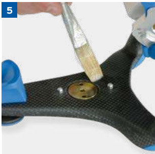
5 Insulate the carbon surface in the area of the adhesive plate by applying a thin layer of petroleum jelly
