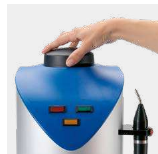
Sealing lid without vulnerable pressure control valve
