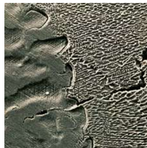
Cracks caused by carbide precipitation in a CoCrMo alloy containing carbon
