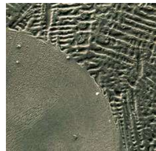
Laser weld without any cracks in a carbon-free CoCrMo alloy
