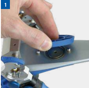
1 Remove model plates, magnets and magnet holders from the upper and lower parts of the Artex articulator
