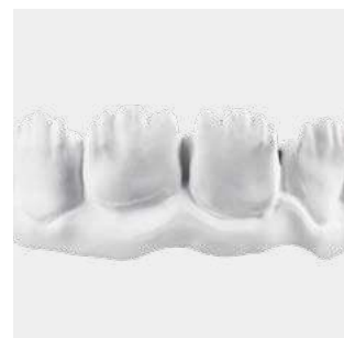
5-axis exterior processing using Ceramill CAD/CAM
