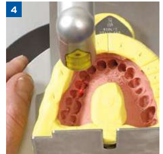
4 Position drilling hole with the aid of the laser beam and initiate drilling procedure
