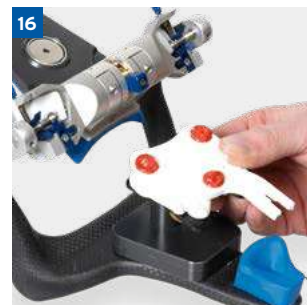
At the dental lab, the transfer table is placed in the articulator or the special mounting articulator used as a plastering device
