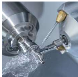
Wet machining of a titanium abutment blank using the "rotary milling" technique
