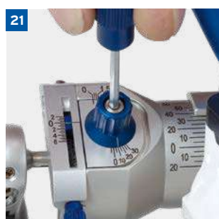
Open the side shift setting screw to open the ISS. Set the anterior guidance pin out of contact
