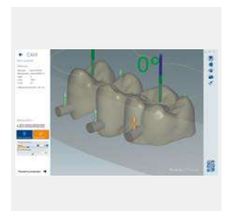
Easy positioning of the connector posts on the designs
