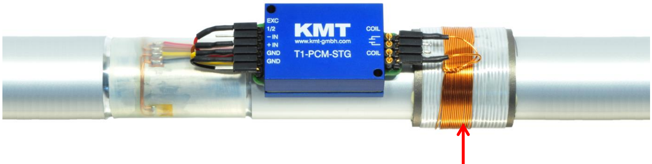
Coil, depends of shaft diameter 5-18 windings of 0.5 CUL wire
